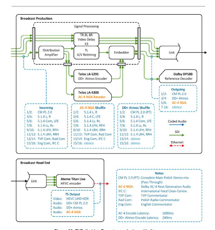
Figure 23. TVP 4k, Live Euro transmission with Atmos
