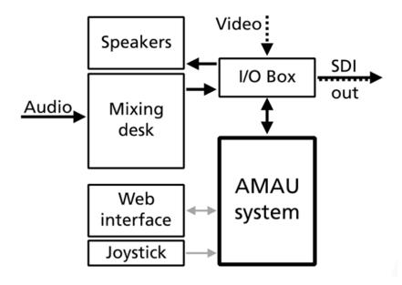
Figure 35. Signal flow of an MPEG-H AMAU System
