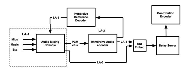
Figure 22. Channel-based Immersive Audio Live Production
