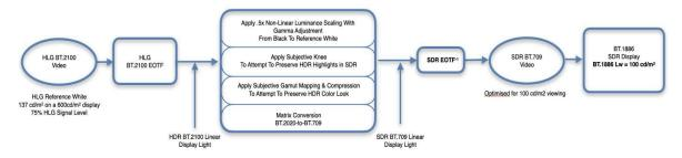
Figure 5: Two Conversion Workflows Through HDR to SDR Down-mapping
