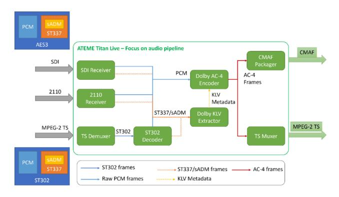
Figure 25. Encoding pipeline using an ATEME Titan Live Encoder
