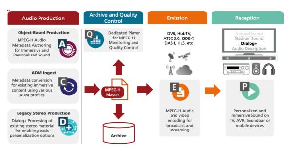
Figure 32. MPEG-H Audio Post-Production workflow (simplified)
