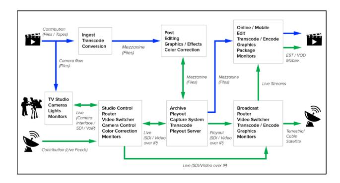
Figure 1. Content Production and Distribution Workflow
