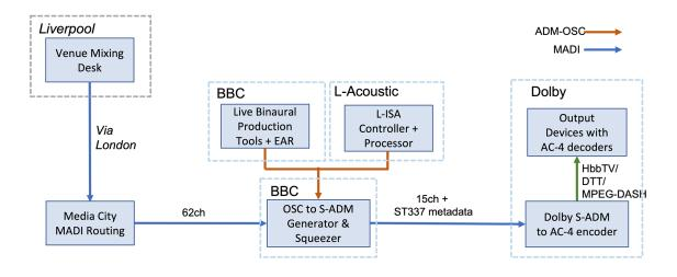
Figure 48: The Test Setup
