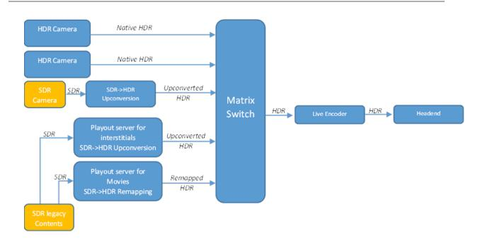
Figure 19. Sample Live Workflow with Mixed Format Source Content
