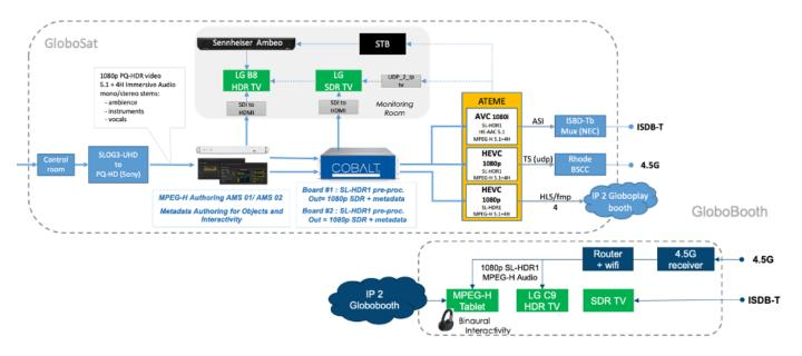
Figure 36. Rock in Rio 2019 setup using MPEG-H Audio
