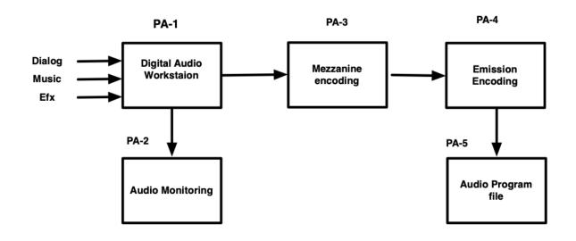
Figure 21. Channel-based Immersive Audio Post-Production
