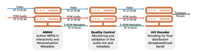
Figure 30. MPEG-H Audio production workflow based on SMPTE ST 2110 (simplified)
