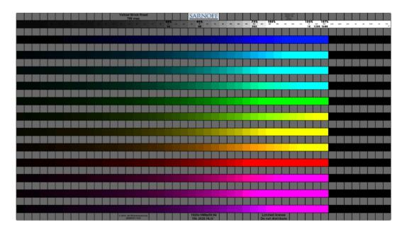
Figure 6. Sarnoff "Yellow Brick Road"© Test Chart (SDR) (courtesy of SRI International)
