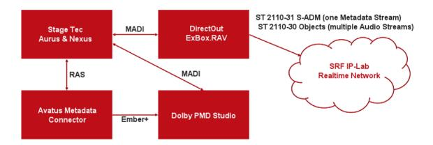
Figure 27. S-ADM setup in the audio control room
