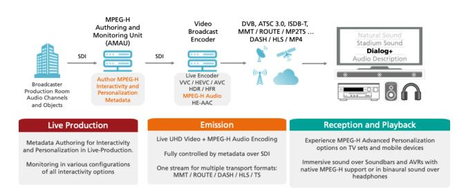
Figure 29. Typical MPEG-H Workflow for Live Productions
