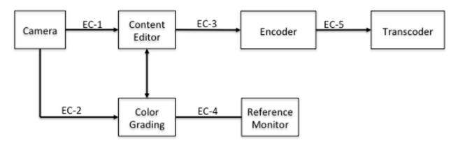
Figure 20. Pre-recorded Content Production Workflow and Interfaces
