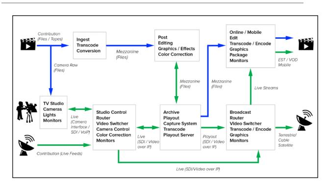
Figure 1. Content Production and Distribution Workflow
