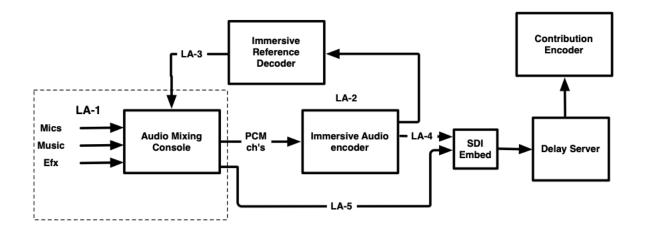
Figure 22. Channel-based Immersive Audio Live Production
