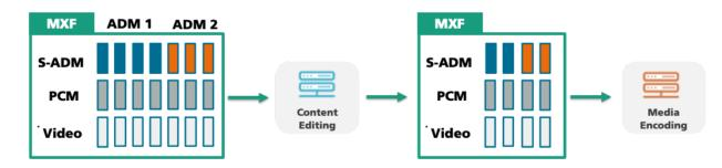
Figure 31. Example of MXF based workflow using ADM metadata
