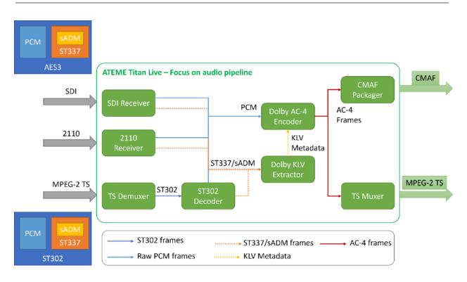
Figure 25. Encoding pipeline using an ATEME Titan Live Encoder
