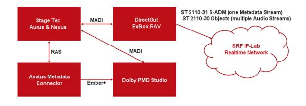
Figure 27. S-ADM setup in the audio control room
