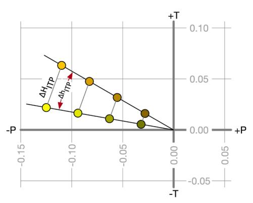
The samples in each color difference pair have the same chroma, for being the same distance from the origin. The hue angle difference  $\Delta h_{ITP}$ , in this illustration from yellow to yellow-orange, is constant for these pairs, but the hue difference  $\Delta H_{ITP}$  increases proportionally to a pair's chroma.
