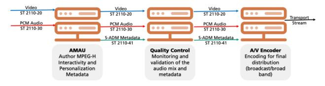
Figure 30. MPEG-H Audio production workflow based on SMPTE ST 2110 (simplified)
