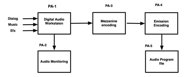
A high-level diagram of a post-production mixing environment for this format is shown below:
