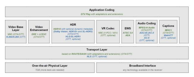
Figure 93. Overview of the TV 3.0 selected technologies for each layer
