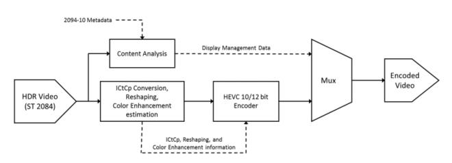
Figure 1. Encoder functional block diagram
