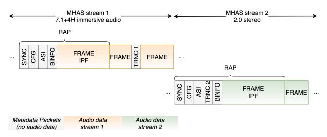
Figure 46. Example of a configuration change from 7.1+4H to 2.0 in the MHAS stream
