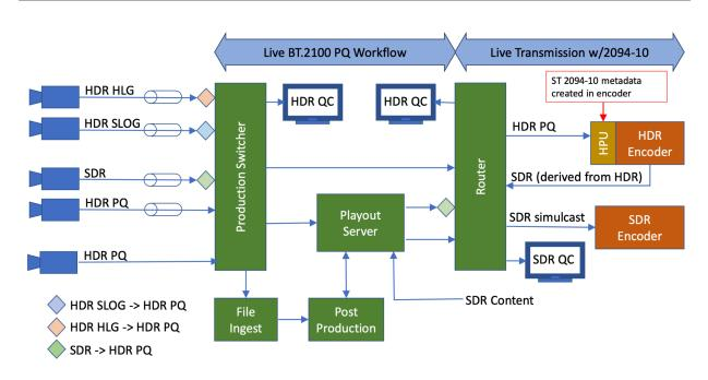
Figure 5. HDR broadcast production facility with BT.2100 PQ workflow- transition phase
