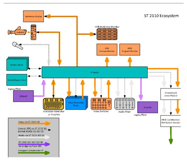
Figure 50. SMPTE ST 2110 live production workflow
