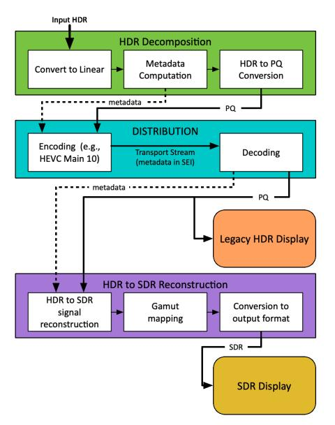
Figure 16. SL-HDR2 processing, distribution, reconstruction, and SDR presentation
