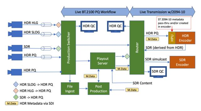
Figure 6. HDR broadcast production facility with BT.2100 PQ workflow- SDI metadata
