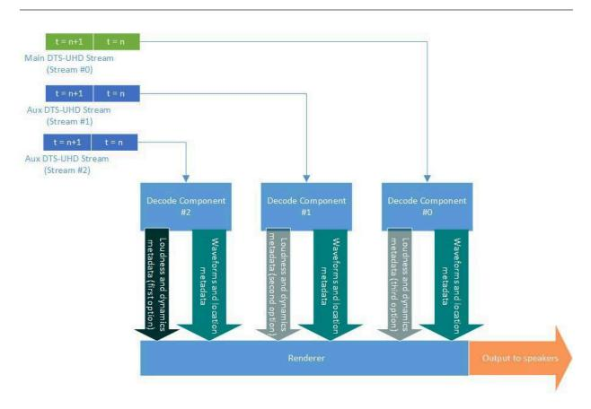
Figure 35. Example of multi-stream decoding
