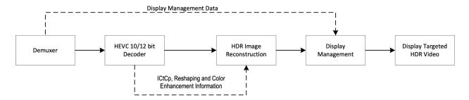
Figure 2. Decoder function block diagram
