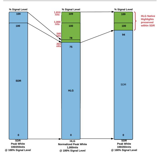
Figure 79. SDR to HLG to SDR Roundtrip Anchor Points
