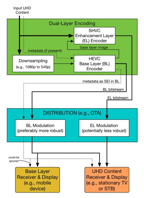
Figure 7. Example dual-layer encoding and distribution
