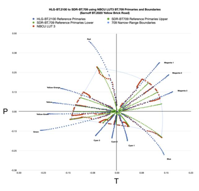
Figure 57. Colorimetric Plot of BT.709 and BT. 2020 Gamuts
