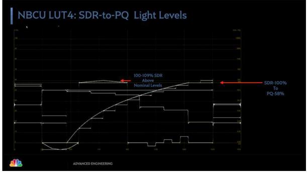
Figure 72. SDR to PQ SMPTE Color Bars with Gray 10% Ladder
