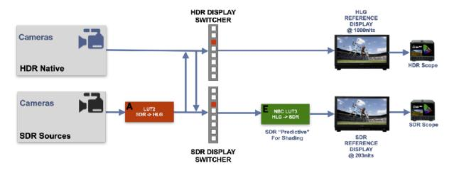
Figure 85. Shading with HDR and SDR Camera Display Switching
