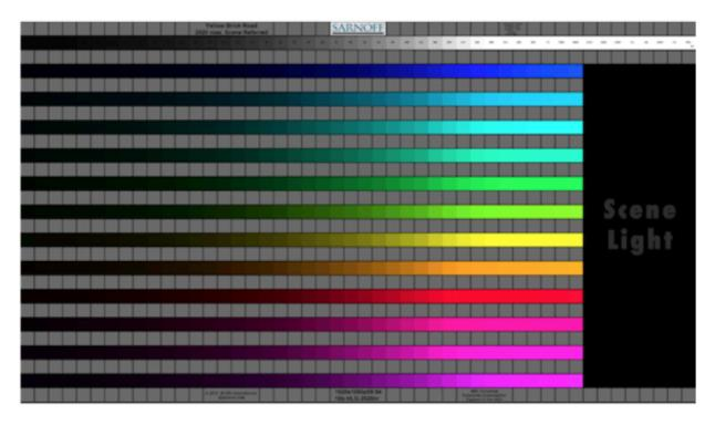
Figure 74. Sarnoff BT. 2020 "Yellow Brick Road" Test Pattern
