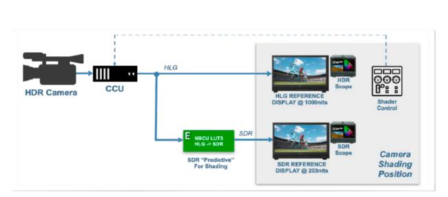
Figure 52. HDR Camera Shading
