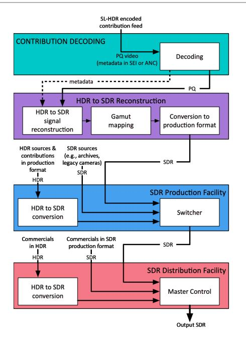
Figure 22. SL-HDR as a contribution feed to an SDR facility
