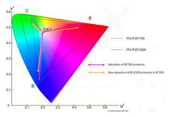
Figure 56. Maximum saturation of the BT.2100 primaries within the BT.709 gamut.
