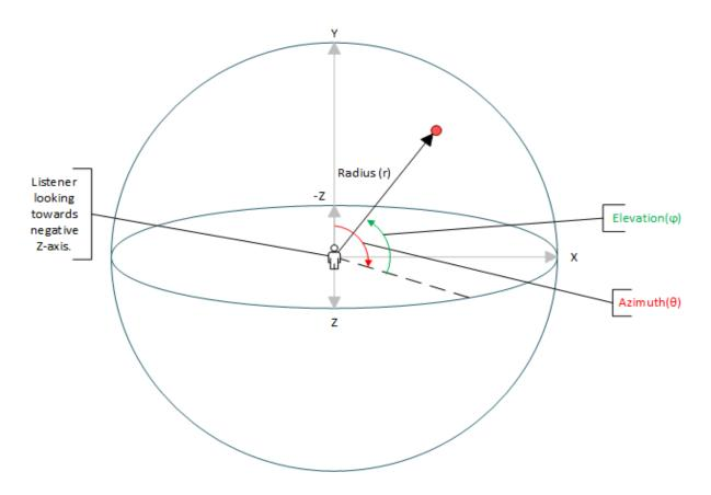
Figure 36. Point Source Object Renderer Coordinate System
