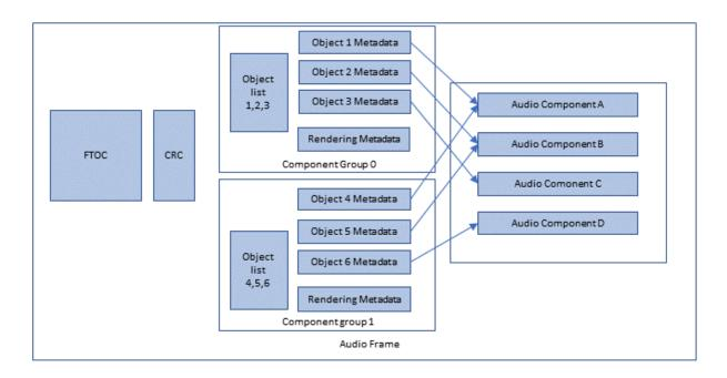
Figure 29. DTS-UHD Audio Frame Structure Example
