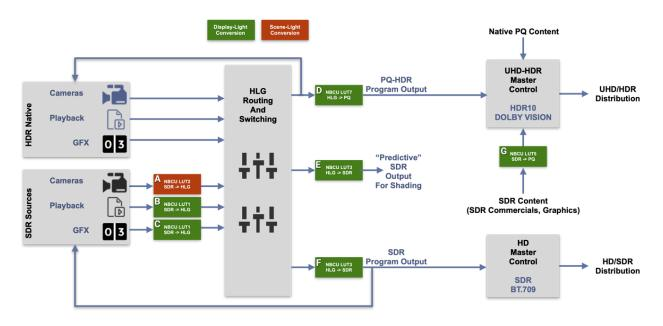
Figure 51. Single Stream Production and Distribution Simplified
