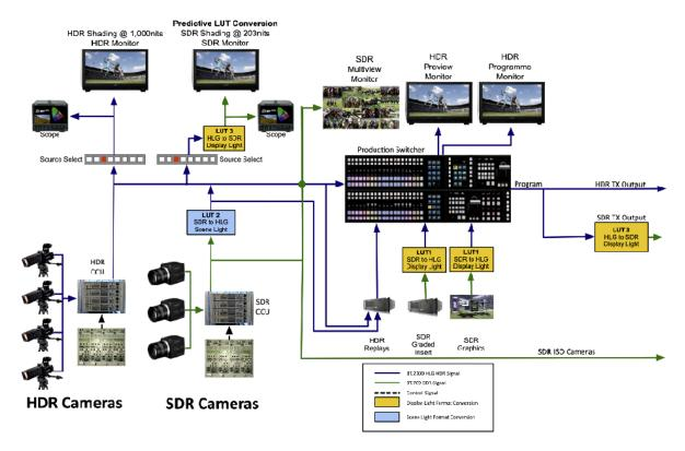
Figure 84. BT.2408 Production Workflow as Modified by NBCU
