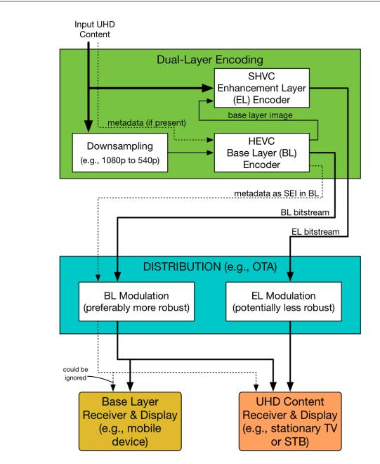
Figure 7. Example dual-layer encoding and distribution
