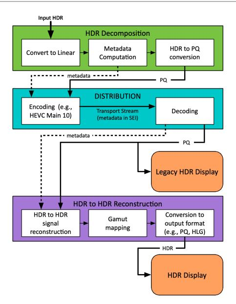
Figure 15. SL-HDR2 processing, distribution, reconstruction, for HDR presentation
