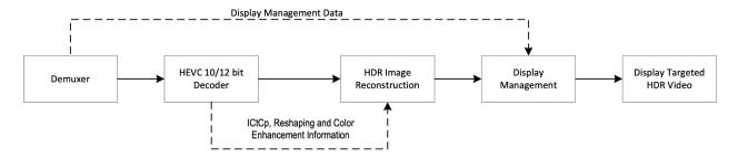
Figure 2. Decoder function block diagram
