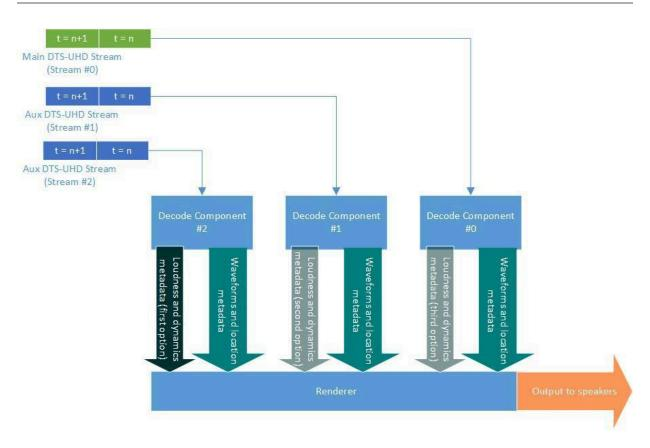
Figure 35. Example of multi-stream decoding
