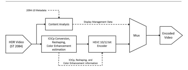
Figure 1. Encoder functional block diagram
