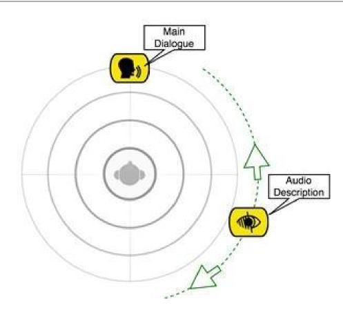
Figure 43. Audio description re-positioning example
