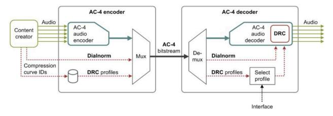
Figure 24. AC-4 DRC generation and application
