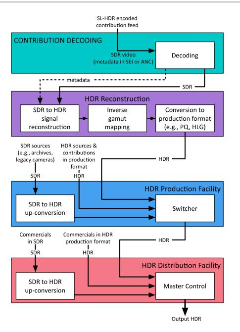
Figure 13. SL-HDR as a contribution feed to an HDR facility
