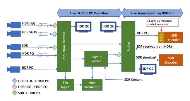
Figure 5. HDR broadcast production facility with BT.2100 PQ workflow- transition phase
