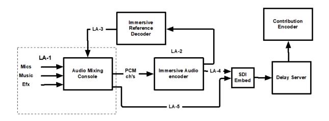
Figure 1. Channel-based Immersive Audio Live Production
