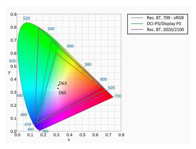
Figure 2. CIE Diagram showing Color System Gamuts, Rec2020, Rec709, P3
