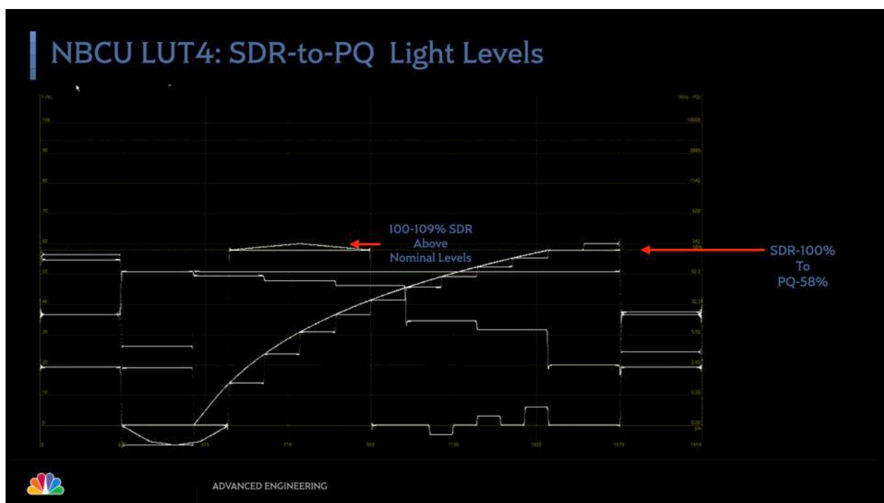
Figure 123 SDR to PQ SMPTE Color Bars with Gray 10% Ladder
