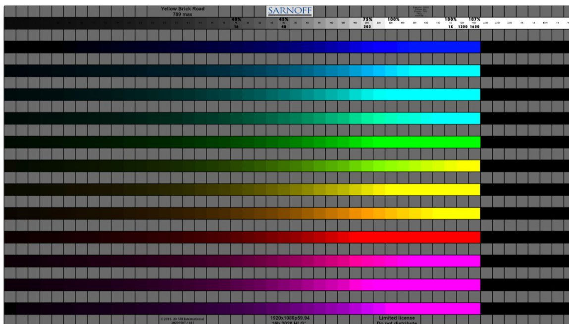
Figure 22 ©Sarnoff "Yellow Brick Road" test chart (SDR) (courtesy of SRI International)
