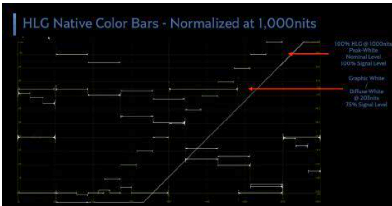
Figure 119 HDR Native Color Bars-Normalized at 1000 nits
