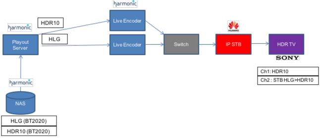
In the demo the STB has access to two video streams, one is encoded in HLG and one is in PQ. When receiving the HLG encoded video, the STB decodes and converts the HLG video stream to PQ format for presentation to the HDR10 based TV set, displaying in HDR10 mode. Switching to the PQ based stream, the STB automatically switches off the HLG $\rightarrow$ PQ conversion, decoding
