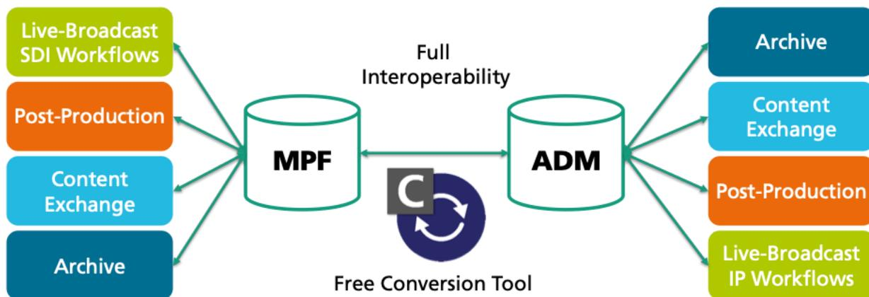
Figure 34. Full Interoperability between MPEG-H Masters and ADM-based workflows
