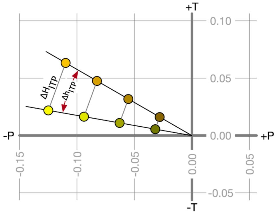
The samples in each color difference pair have the same chroma, for being the same distance from the origin. The hue angle difference  $\Delta h_{ITP}$ , in this illustration from yellow to yellow-orange, is constant for these pairs, but the hue difference  $\Delta H_{ITP}$  increases proportionally to a pair's chroma.
