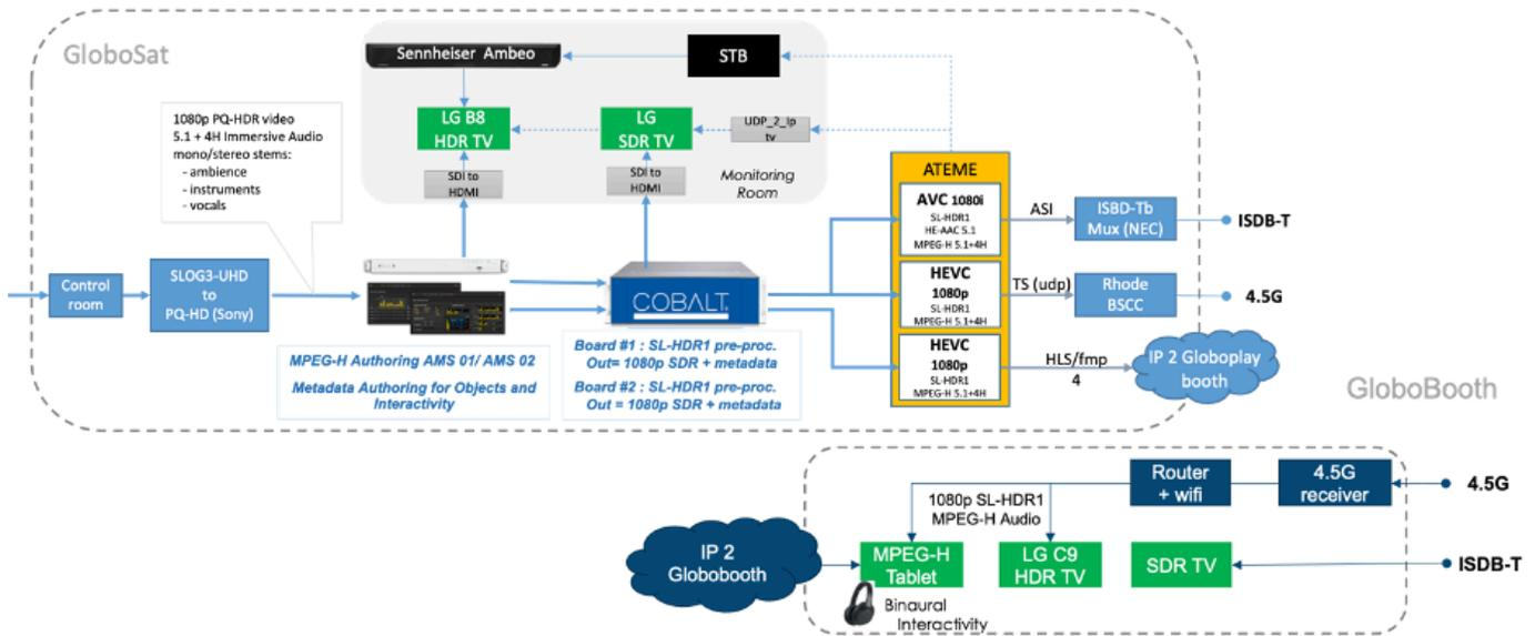
**Figure 36. Rock in Rio 2019 setup using MPEG-H Audio**
