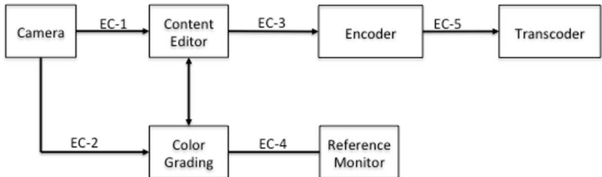
**Figure 20. Pre-recorded Content Production Workflow and Interfaces**
