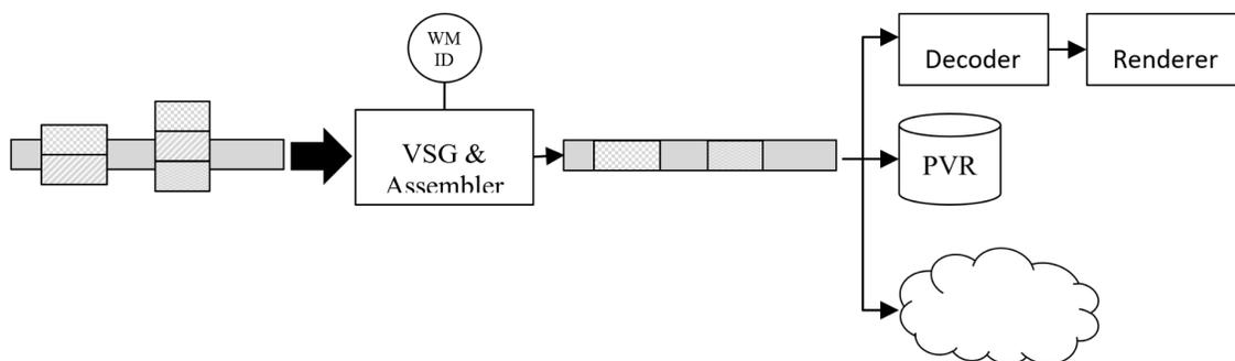
**Figure 10. Watermark Embedding Using a Unique Variant Sequence**
