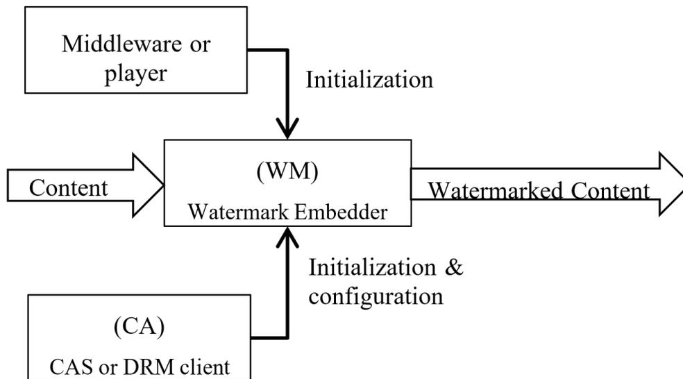
**Figure 7. One-Step Watermark Performed on the Client Side**
